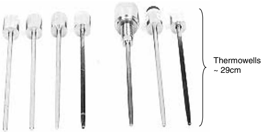
Fig. 4.10. Examples of RTD thermowells of the type used in nuclear power plants
